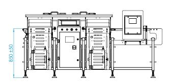
The combination unit is fitted with a Fortress Technologies detector head, which can be supplied with sizes to suit most standard applications and uses powerful Digital Signal Processing technology and high sensitivity levels to ensure the detection of the smallest ferrous, non-ferrous, and stainless-steel contaminants.
